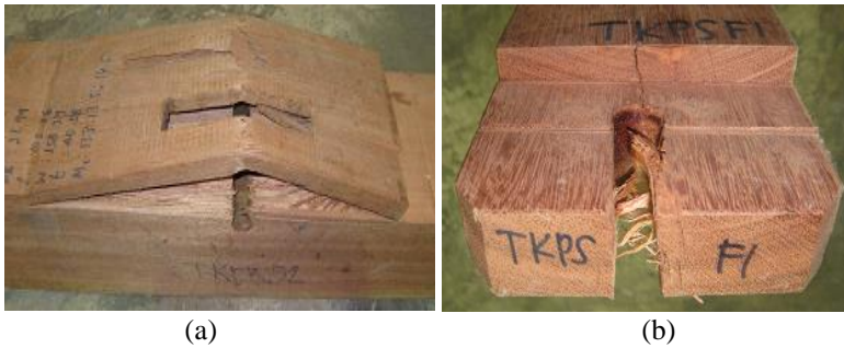
Figure 4: Mortise and tenon failure; (a) side of the mortised-member failed in major failure – heavy splitting or shearing-out of the mortise, and (b) tenon-end failed in major failure – heavy splitting or shearing-out of the tenon end
