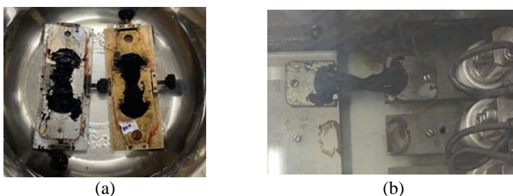
Figure 4: (a) Bitumen filled briquettes conditioned in 27 °C water bath, and (b) Briquettes removed from mould and hooked into machine
